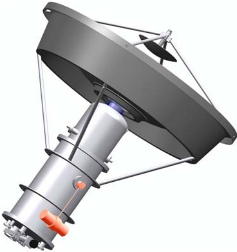
Figure 6. The optics and the cryostat
