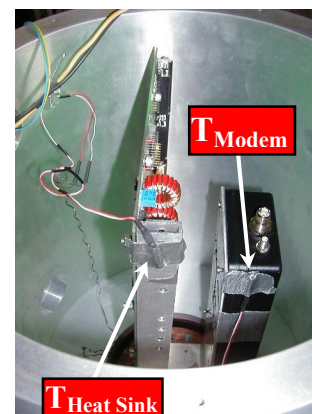
Fig. 6. MSITel and NAL modem in the test vacuum-chamber. The Pt100 temperature sensors are also shown.
