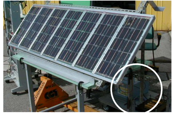
Fig. 5. The solar panel (SP) prototype during test connected to the rechargeable batteries (white-circled in the right down corner).
