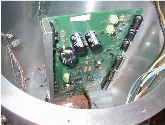
Fig. 10. The SPSys PCB in the vacuum chamber. The heat sink for the active components is also shown.
